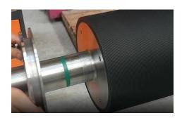
**EOS Sleeves** is not a product, it is a **SYSTEM that allows immediate and independent replacement of rubber coating,** ensuring the continuity of the production line, now also **the GLUE line.**
